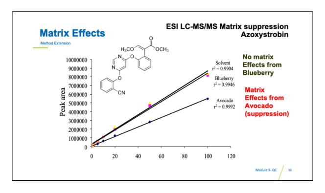
This slide is a specific example of the same pesticide analyzed in blueberry and in avocado. The solvent and blueberry matrix lines are equivalent, which means that there is no matrix effect. However, the avocado matrix calibration curve is suppressed.
