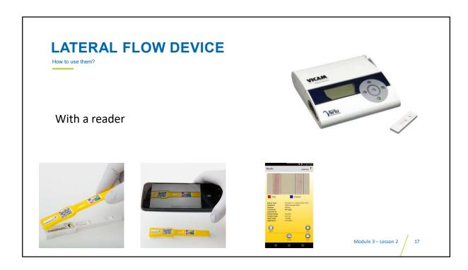
For qualitative measures, an LFD reader will be mandatory. Some producers have dedicated equipment (like the Vicam reader), others have developed alternatives. For example, some smartphone are now regularly used as reader by using their camera. In this case, the results are display on the screen of the phone.
