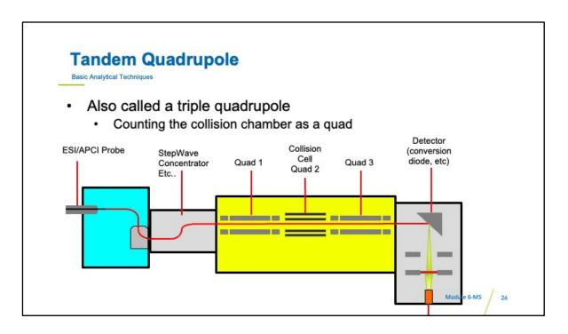
The most widespread implementation for the analysis of food contaminants by LC with a mass spectrometer is the tandem quadrupole. As mentioned earlier, some vendors call it a triple quadrupole as they count the collision chamber as quadrupole 2. It is also not uncommon for these to be called quads, rather than quadrupoles.
