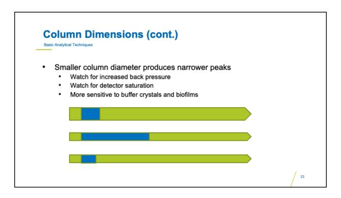
I wanted to illustrate in a very simple schematic what happens when you move from a wide to a narrow column. First, if you try to inject the same volume of sample, it will occupy a much larger proportion of the length of the narrow column. This means that you only have what is left on the right hands side to separate the analytes contained in that sample. Consequently, we normally reduce the volume of sample when we move to a narrower column.
