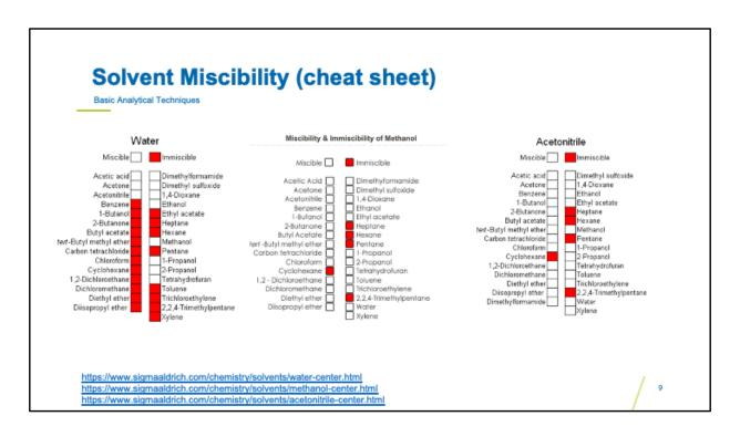
These are more examples of graphical representations of this miscibility and I like to just print these types of graphical representations and posting them either on the side of the instrument or close to the mobile phase preparation area in the wet lab to remind ourselves of what can be mixed and what requires a transition phase.
