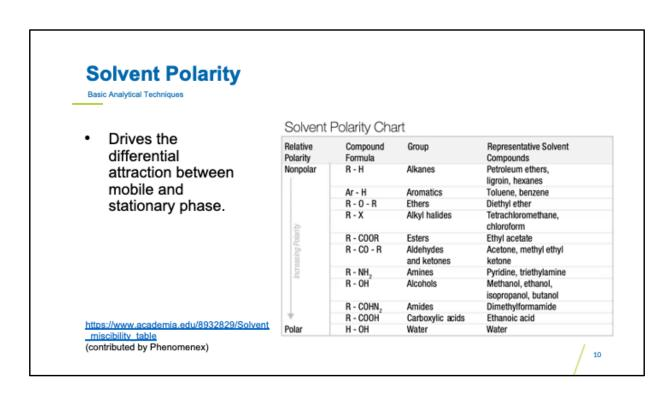
The next parameter is solvent polarity. It is the differentiating factor that either carries analytes through the column quickly or not. In other words, the difference in polarity determines whether the attraction is greater between the analytes and the stationary phase or between the analytes and the mobile phase.
