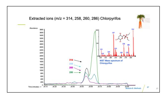
Now we have the mass spectrum on the right and the three chromatograms from the single reaction ion monitoring for m/z = 314, 258, 260, 286.
