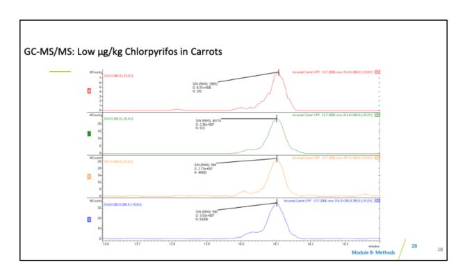
So we go to GC-MS/MS: for the same sample, where we are looking at the transitions: 314>286, 314>258, and 314>250, and 197>169. All of them have very high S/N ratio and no interference.
