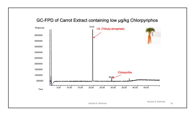
In this second example, we are looking at GC-FPD of Carrot Extract containing low concentration of Chlorpyrifos, another organophosphate pesticide.
