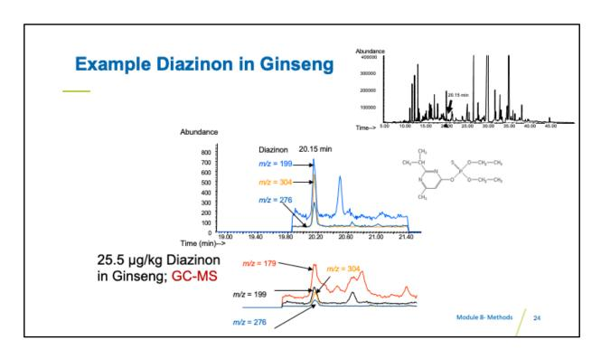
In GC-MS, we have a peak in the chromatogram on the top right at 20.15 min, and we see the overlapping peaks of our internal standard and ions for diazinon.
