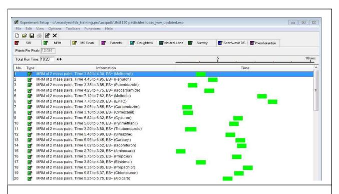
Figure 5: Waters' MassLynx window illustrating the period of time during which data acquisition is performed for a list of pesticides in an MRM method.
